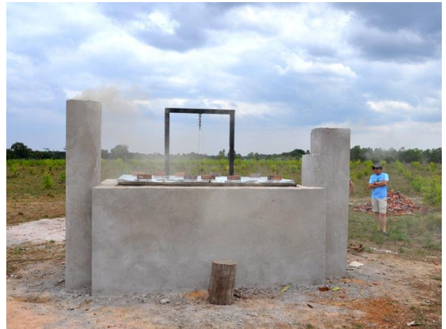
Adams Retort based on pyrolysis principle which we built at La Pedregoza for Biochar production.
